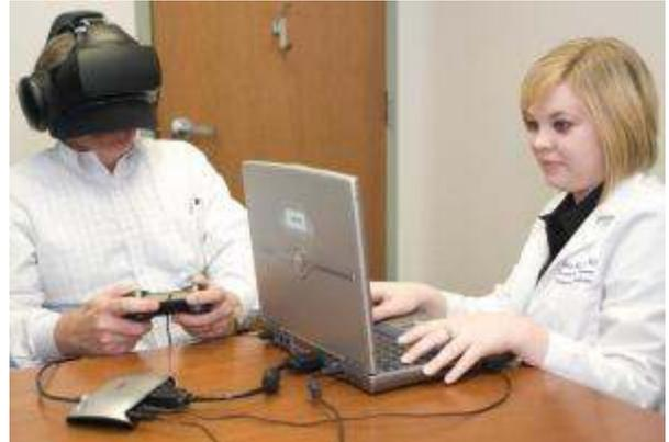
*The DETECT system includes an LCD display in a visor with an onboard dedicated computer, noise reduction headphones and an input device (controller). The display projects the visual aspect of the test and the headphones provide the verbal instructions. (Credit: Image courtesy of Georgia Institute of Technology)*
